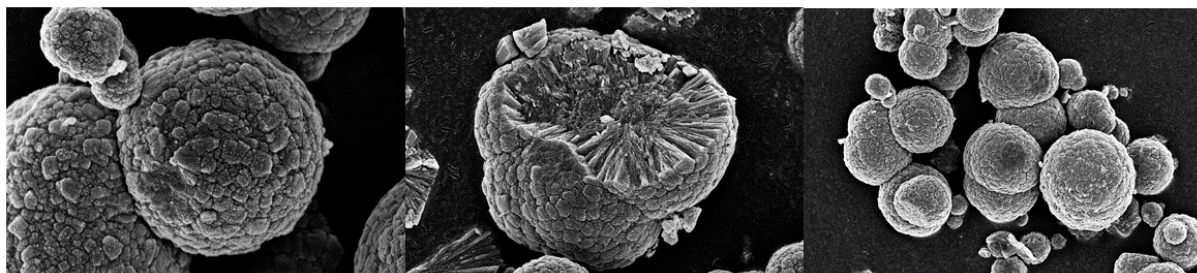
Figure 1.8. SEM images exemplifying the spherulitic ZnS particles. 61
