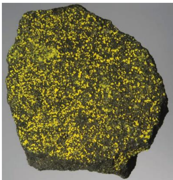
Figure 3.4. Black coffinite rock with a ~1 mm uranyl sulfate yellow coating. 65
