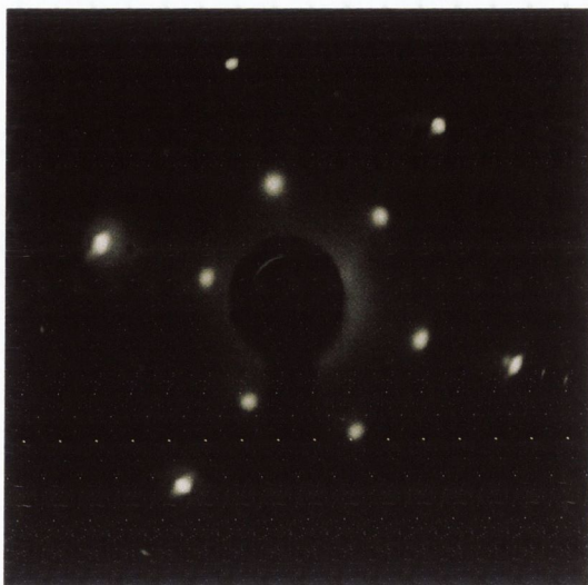
Figure 4.4: The p(2 \times 2) LEED pattern due to 0.25 ML of oxygen adsorbed onto the Mo(110) surface. E_{beam} = 57 eV.
