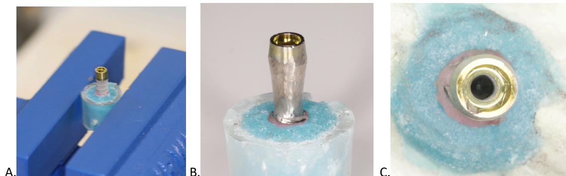
Figure 8: Photographs showing the placement of an implant pre-IP in a tabletop vice grip, B. Sweden & Martina® implant after IP and C. Presence of a notch on the internal surface of the tabletop implant
