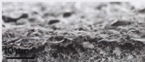
Figure 6.19: SEM image of the cross section of a polymer-composite film deposited on a PVDF membrane.
