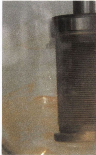
Figure 5.8. Photograph of dye radiating outwards from the side of the basket at 50 rpm. Three distinct streams of radiating dye are visible here: one above the lower lip, one below the upper lip and one almost midway up the side of the basket.
