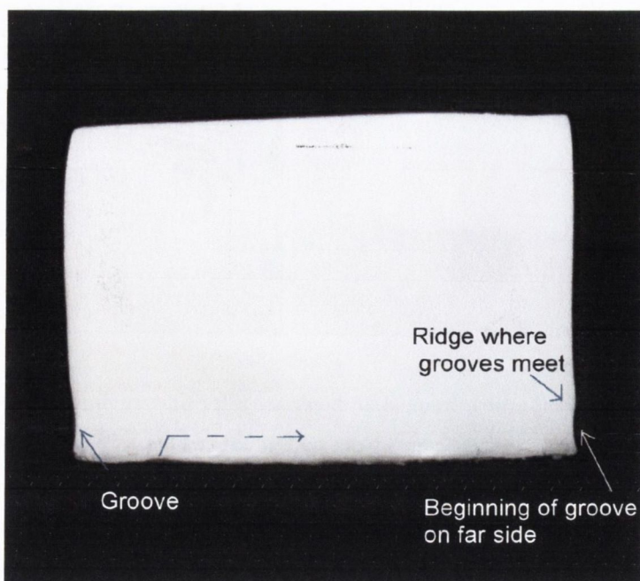
Figure 3.11. Photograph of the 8.5 mm benzoic acid compact after dissolution for 1 hour in position 1, in 900 ml 0.1M HCl in the paddle apparatus at 50 rpm. The left hand side of the image was facing the centre of the vessel. The groove on the side of the compact facing into the fluid flow is facing the front, and the end of this groove, the diagonal ridge and the beginning of the groove on the far side of the compact are also visible here.
