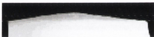
Figure 4.6. Photograph of a benzoic acid compact after 5 hours dissolution in the central position. The “peak” which developed can be seen in the centre of the top planar surface.
