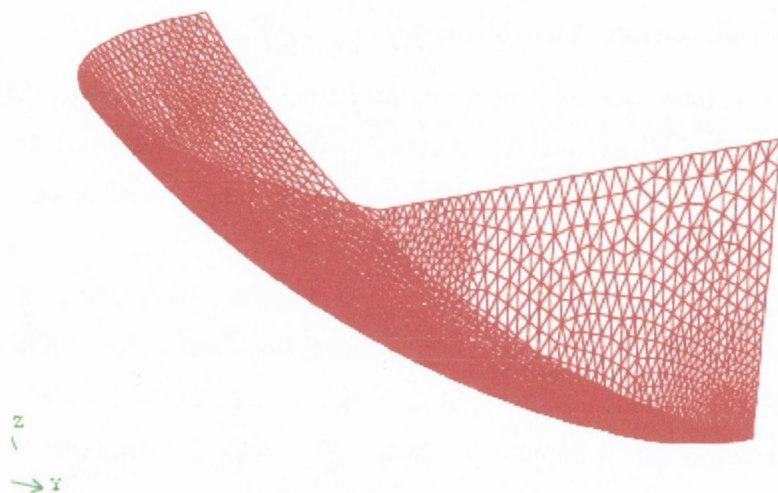
Figure 2.3. Source face and side face of one of the lower quadrants in the paddle apparatus illustrating the continuous effect of the size function through the attachment entity.
