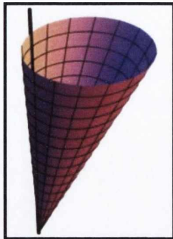
Figure 1.6: The skewed cone traced out by the Poynting vector \mathbf{S} for a single ray aligned with the optic axis (solid black line). The skewed cone has semi-angle A as defined in Eq. (1.20). The colour gradient is for clarity only.
