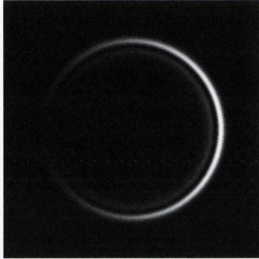
Figure 1.13: The intensity profile at the FIP produced by a linearly polarised incident Gaussian beam, found using Eq. (1.75) with \phi = 0 . The parameter \rho_0 = 20 , and the image has dimensions 3\rho_0 \times 3\rho_0 .
