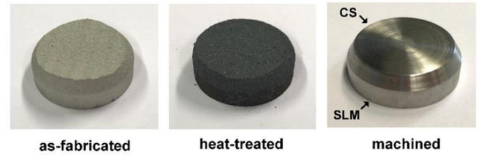
Figure 13: Photos of the CS/SLM 316L stainless steel part manufactured from as-fabricated state to final machined state
