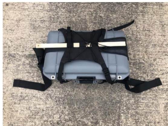
Figure 12 The LI – 7810 CH 4 /CO 2 /H 2 O Trace Gas Analyser (LI-COR)
