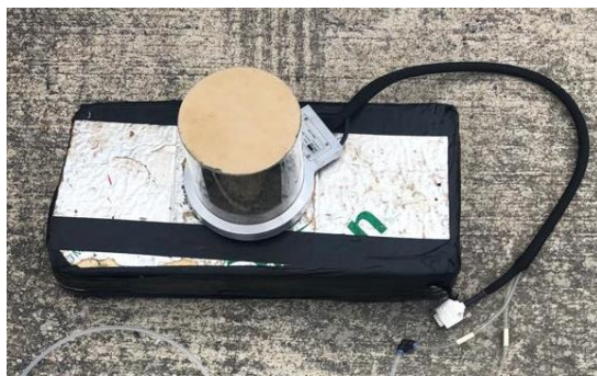
Figure 11 The chamber placed on top of the collar which has been inserted tightly into a polystyrene insulation board which floats.
