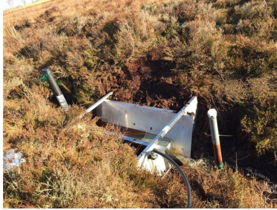
Figure 5 Installed flume in CL Upper natural stream
