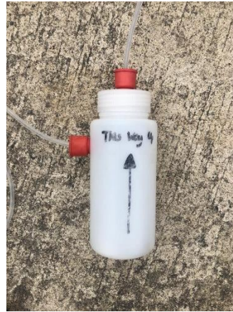
Figure 10 The water trap connected to the chamber and analyser.
