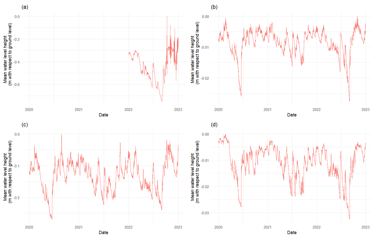
Figure 52 The water level data (m with respect to ground level) for CL marginal (a), sub-marginal (b), central ecotopes (c) and sub-central (d) ecotopes.
