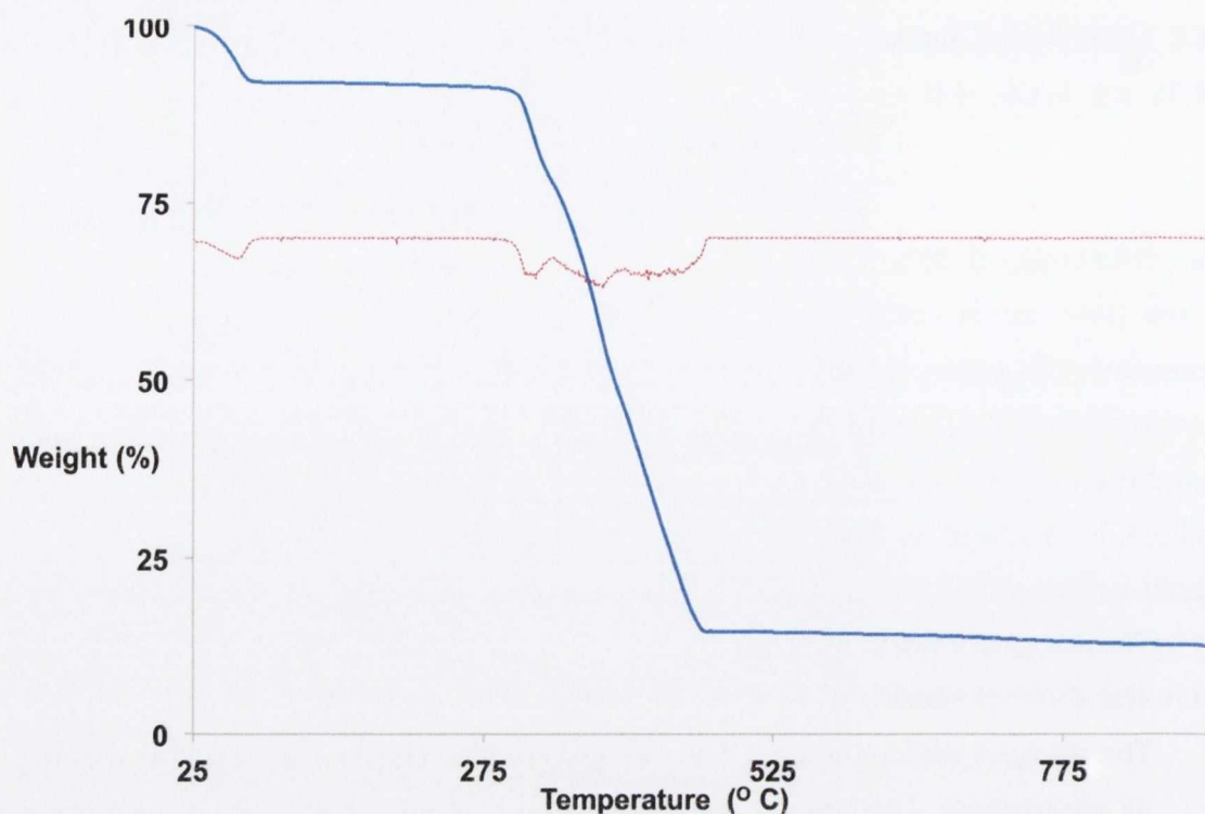
Figure 3.26: TGA curve for 11 . Recorded in an air atmosphere from 25 °C to 900 °C. Heating step was set to 5 °C/minute.
