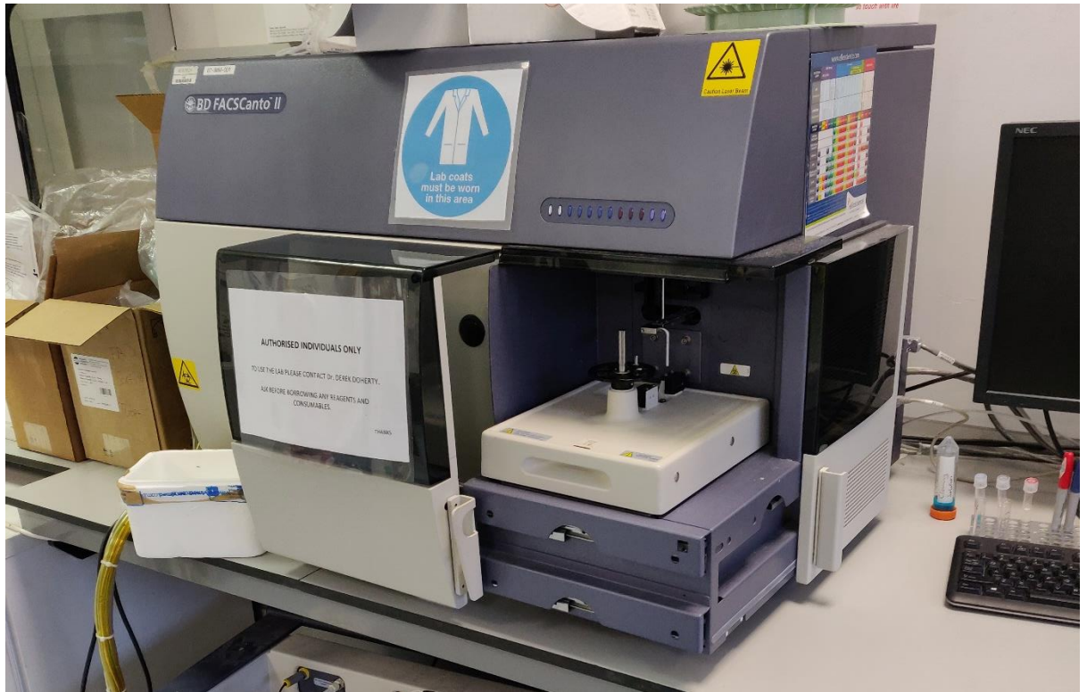
Figure 2.2: BD FACSCanto™ II flow cytometer used for flow cytometry analysis.
