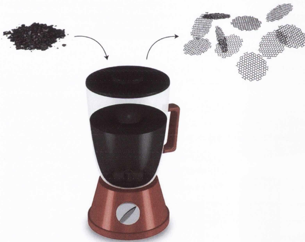
Figure 2.12: Graphic demonstrating exfoliation of nanosheets through shear exfoliation.
