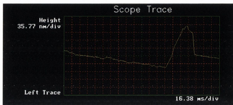
Fig. 28 Example of a single unlevelled trace AFM image of a cut made in a polymer film of MEH-PPV which was spin-coated from a 15 g/l chlorobenzene solution at a spin speed of 1500 rpm.
