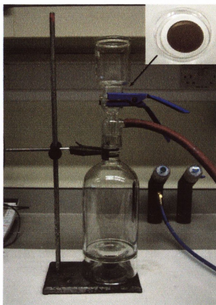
Figure 2.4: Vacuum filtration apparatus for the production of nanostructured films.
