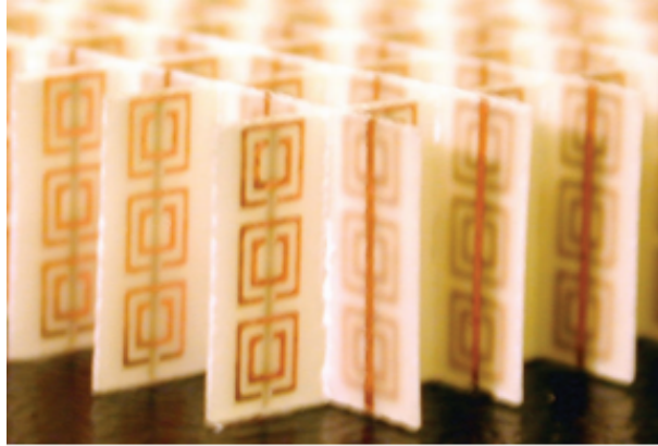
Figure 2.5: A periodic array of copper split-ring resonators on fibre glass circuit board [1].
