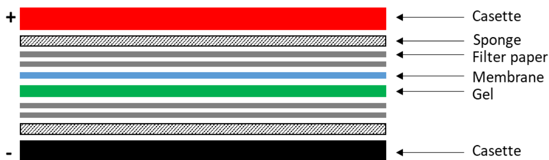
Figure 2.2. Wet transfer layout. Current ran from the anode to the cathode.
