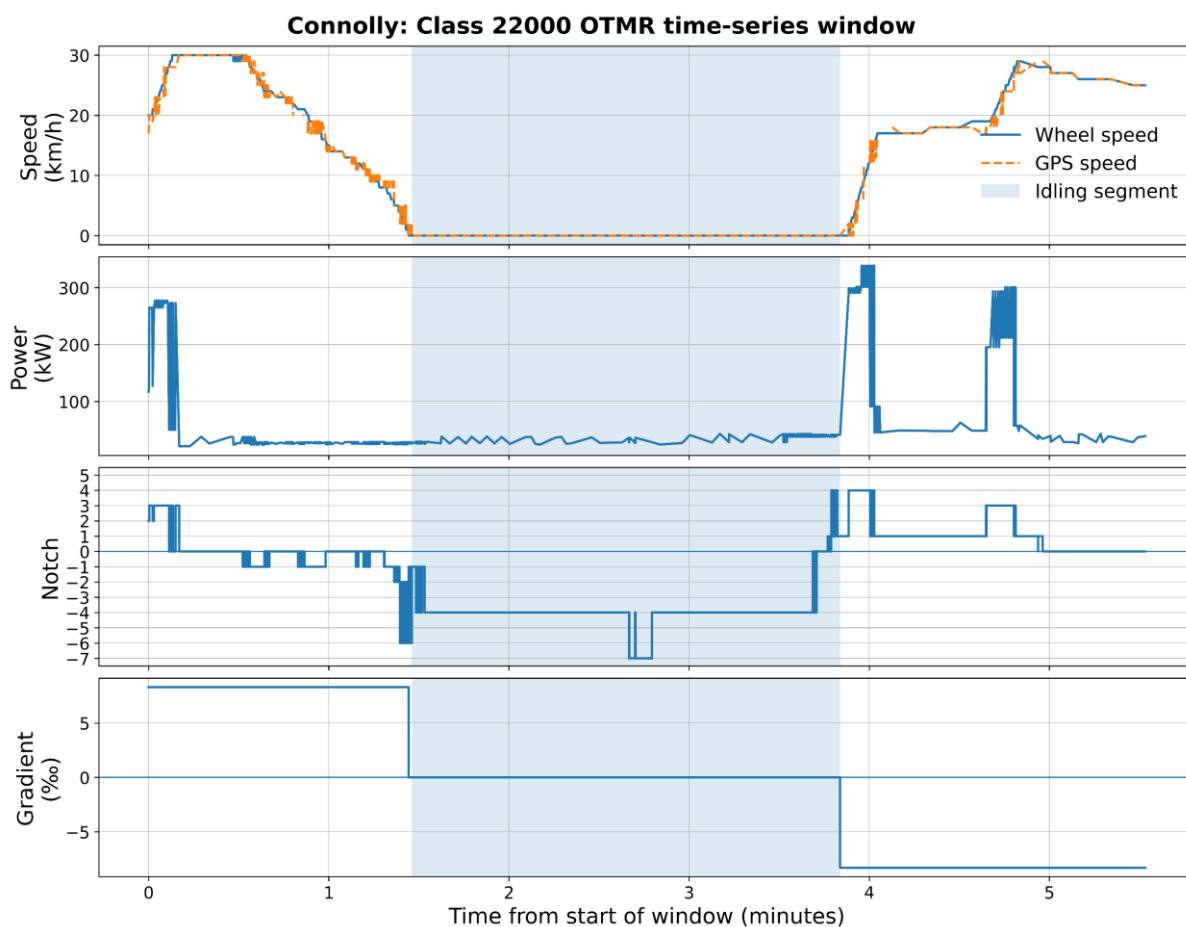
Figure 4.3 Connolly Class 22000 OTMR time-series window showing wheel speed, GPS speed, engine power, notch position (Positive notch values indicate power notches, while negative notch
