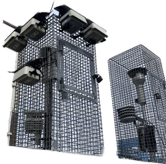
Figure 3.5 Low-cost monitors co-located with the Ringsend EPA station (reference site 1)
