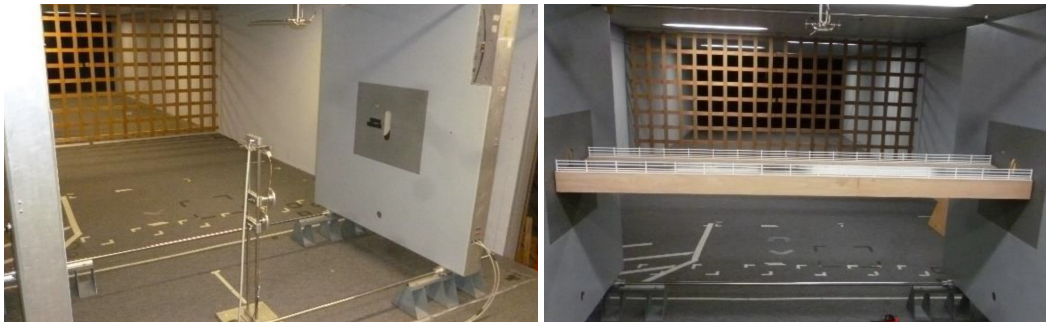
Figure 3.9. Test setup for the Clyde Bridge deck model (Carusone & Flamand, 2022)
