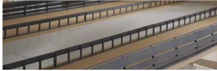
Figure 3.19. Wind shielding and traffic barriers installed on the Narrow Water Bridge model (Svend Ole Hansen ApS, 2023)
