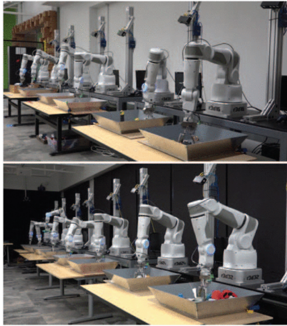
Figure 2.11: Large scale data collection setup used to create the Google Grasp Dataset [190]. 14 robots collected 800,000 grasp attempts
