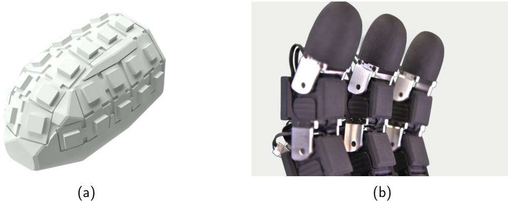
Figure 2.7: uSkin curved product offered by xelarobotics, specifically designed to be used as the fingertip for the Allegro robot hand [127]. (a) shows a rendering of the sensor and (b) shows a photo of uSkin deployed on the gripper
