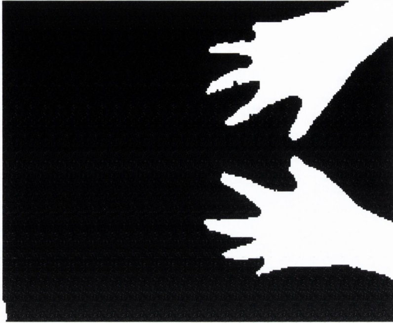
Fig. 3-16 Grey threshold value scaling factor set too high, portion of fingers lost in monochrome conversion
