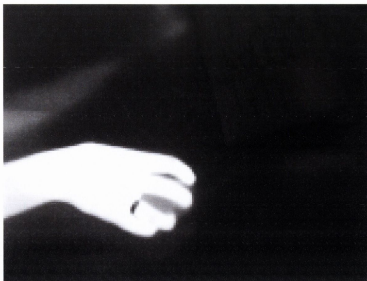
Fig. 4-10 Typical infrared temperature profile converted to black and white image based on temperature
