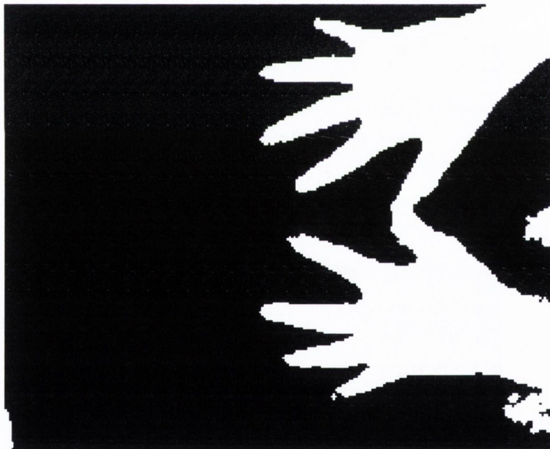
Fig. 3-9 Processing Stage 3: Image is converted to monochrome using the grey threshold value
