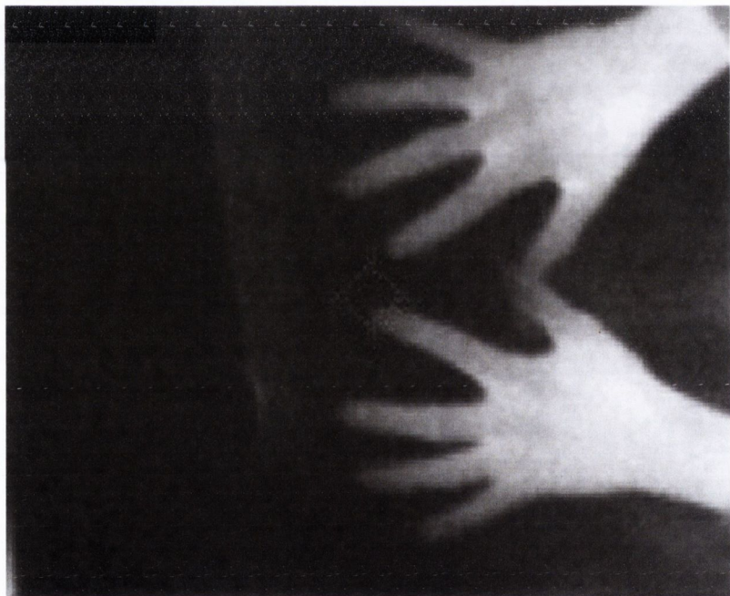
Fig. 3-7 Processing Stage 1: Image cropped, crosshairs, temperature bar, FLIR logo and emissivity value removed
