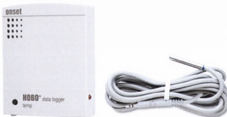
Fig. 3-20 Onset HOBO U12 Data Logger and PT-100 Sensor (www.onset.com, 2012)
