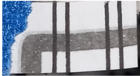
Figure 42. Printing of SnSe 12 mg/ml on paper (grey). The electrodes of graphite ink are 2 mm apart (black).
