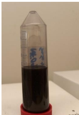
Figure 27. Photograph of a SnSe dispersion obtained by tip ultrasonication.
