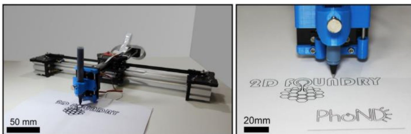
Figure 36. Pen plotter to draw the pattern of the 2D Foundry on paper. Picture credit: Reference 103.
