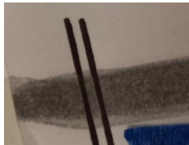
Figure 48. Printing of PtSe 2 16 mg/ml on paper (grey). The electrodes of ink graphite are 2 mm apart (black).
