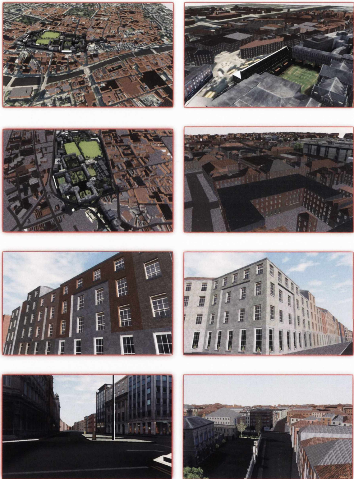
Figure 3.24: City generated in real-time. Procedural building models are integrated with user created 3D CAD models of the Trinity College Campus. By utilising GIS data, buildings may be placed on top of satellite imagery.
