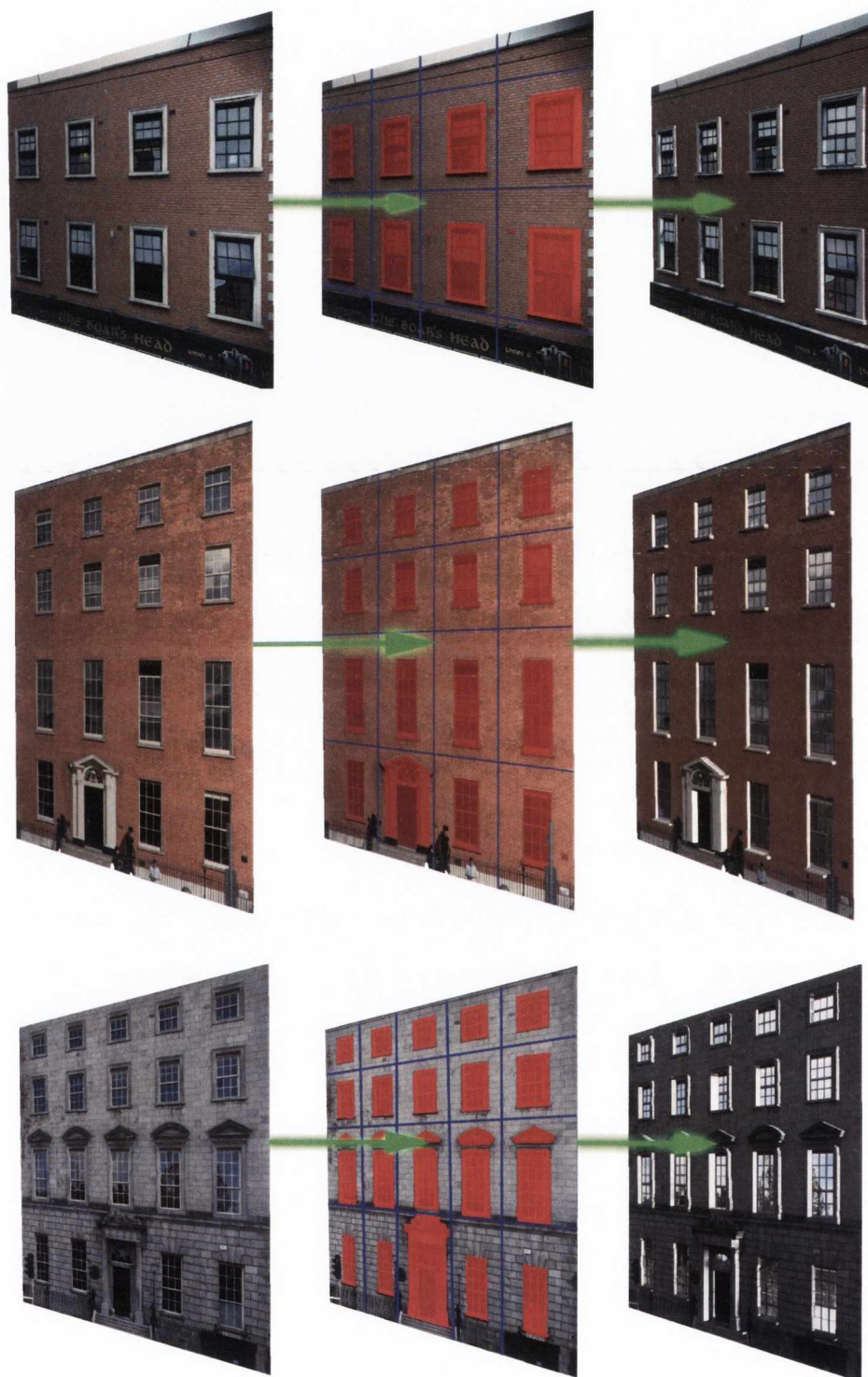
Figure 4.21: Results of applying our segmentation method to three different facades. Left: Input rectified photographs. Middle: Segmented facade elements. Right: Resulting 3D facade models after manual depth adjustment. Shaders were added to the windows to provide reflection effects.
