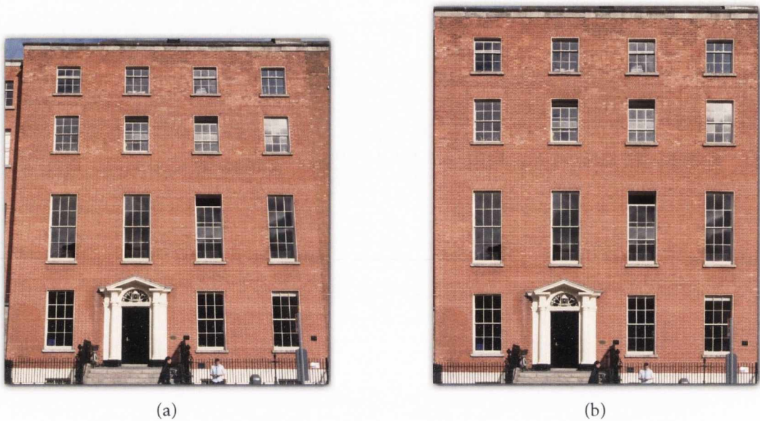
Figure 4.2: (a) Input facade image has perspective distortion. (b) Rectified facade image.
