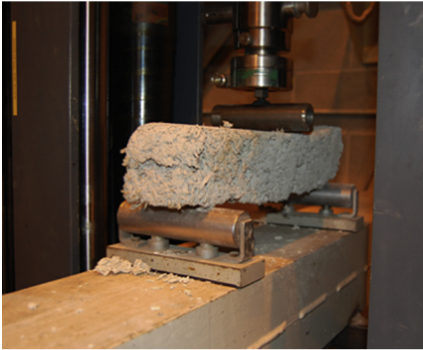
Fig. 8. Typical deflection of hemp-lime concrete in bending.
