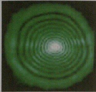
Figure 2.2: Interference ring pattern produced by light phase modulation.
