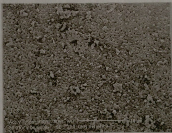
Figure 4.22: High magnification SEM micrograph of the etched surface of the 60/40 unsaturated polyester based PDLC composition after curing.
