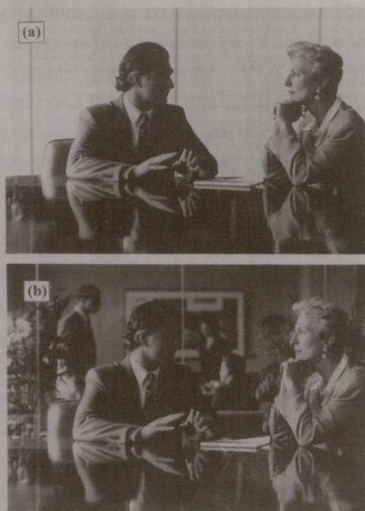
Figure 1.1: A demonstration of a PDLC privacy window made with 3M TM Privacy Film. The laminated glass allows total privacy at a flip of a switch. The glass changes from a milky white appearance (a) to a transparent appearance (b).
