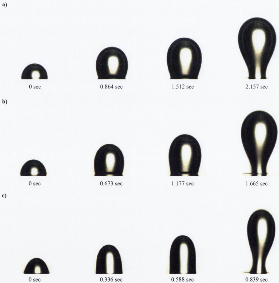
Figure 7.1: Photographic sequence of bubble growth under the influence of an electric field strength of (a) 0 (b) 0.4 and (c) 0.8 kV/mm.
