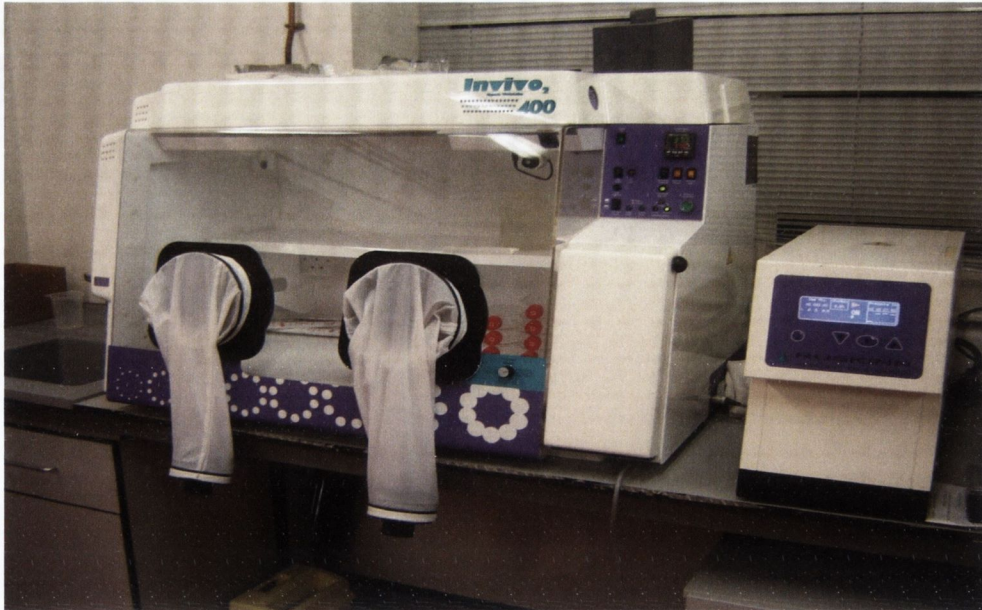
Fig 2.1 The hypoxia chamber. The Invivo 2 400 Hypoxia Workstation with Ruskin hypoxia gas mixer. The Machine provides accurate control over O 2 (0.1%- 20.9% in 0.1% increments) and allows the transfer of samples and access to the environment without affecting stability.
