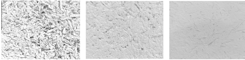
Fig. 3. Surface finishes of (left) unfinished hemp-lime concrete, (middle) 1:1.25 lime-hemp render, (right) 2:1 lime-hemp render.
