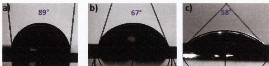
Figure 5.9: Water contact angle measurements of a) bare graphene, b) low density 1 on graphene and c) high density 1 on graphene.
