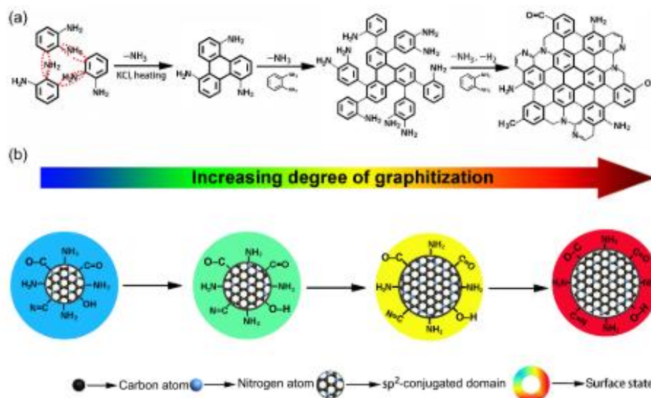
Figure 1.15, A formation mechanism (a) and PL mechanism (b) for CDs with tuneable PL emission. 123
