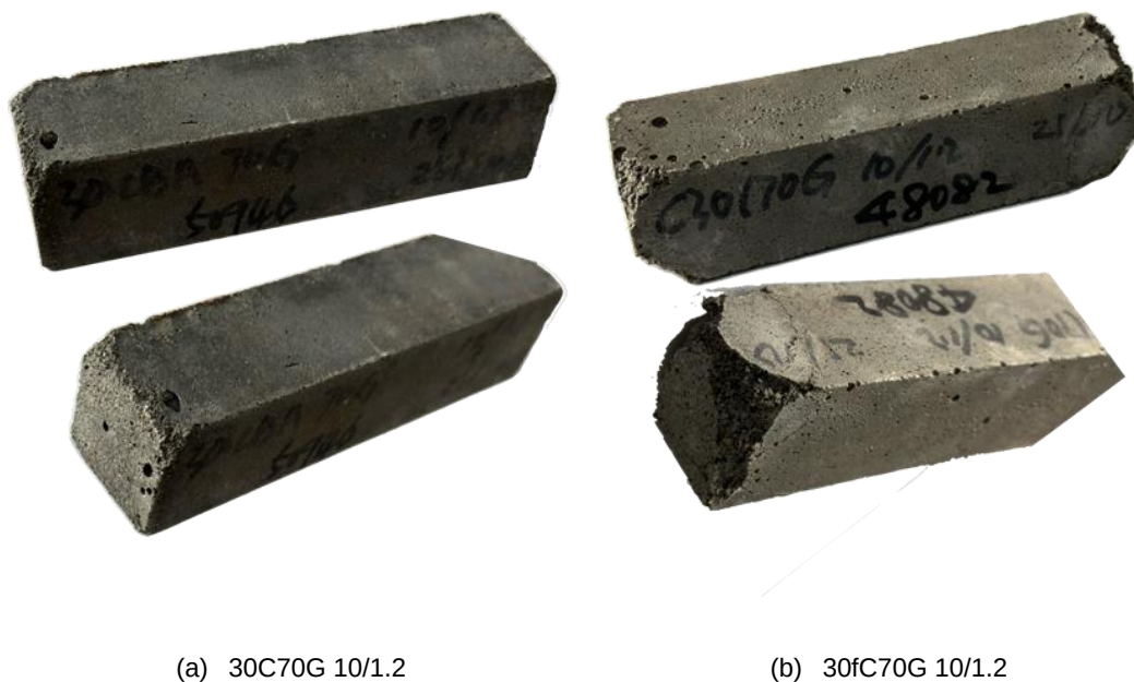
Figure 8-4 Photographs of CBA-based two-part geopolymers after sulphate attack.
