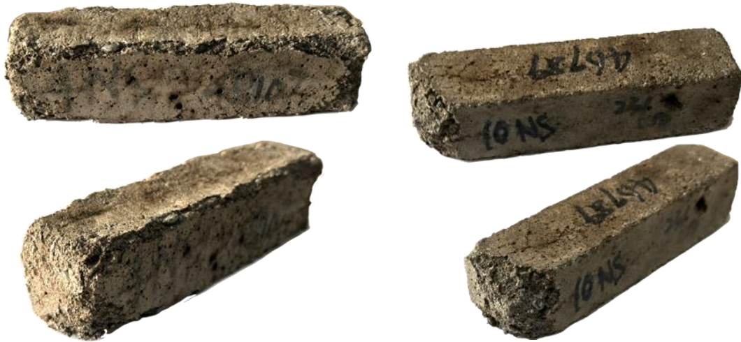
Figure 8-7 Photographs of OBA-based, one-part geopolymers after sulphate attack (left: 40A60G4Cs, right: 40A60G10Cs).
