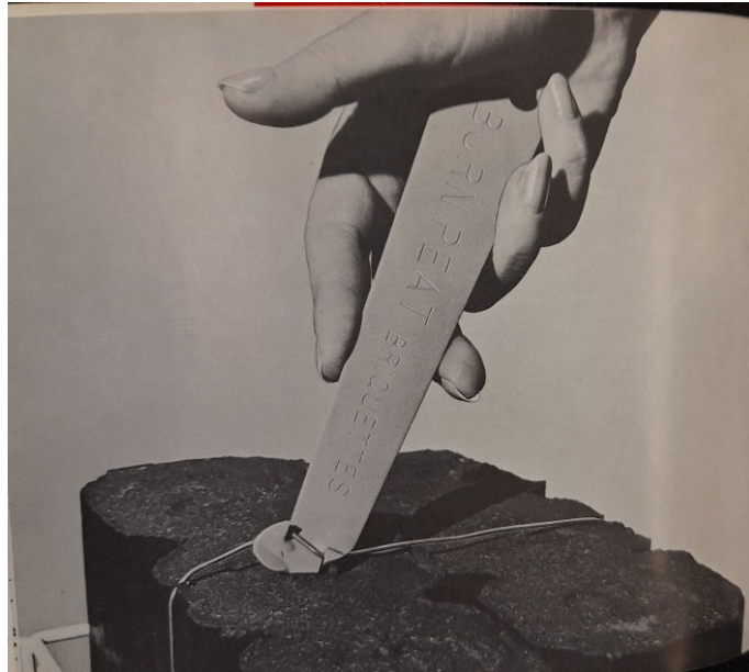
Figure 4.10 Metal strap-breaker, in Bord na Móna “Annual Report.” (1962-63), 8.
