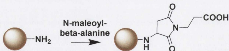
Figure 2.10: Schematic of carboxyl functionalisation using amino-maleimide 'Click' chemistry
