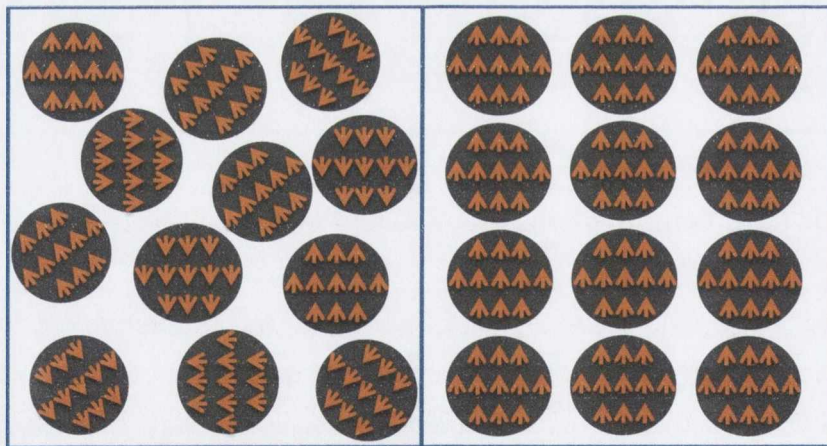
Figure 1.3: Schematic of superparamagnetic materials, with magnetic domains (orange) and their alignment in the absence of (left) and presence of (right) a magnetic field
