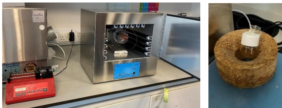
Figure S7.2: Continuous flow system within a 110 V UV oven (Scanlan Laboratory, Trinity Biomedical Sciences Institute, Trinity College Dublin, 152-160 Pearse Street, Dublin 2, Ireland). Investigation of the radical mediated thiol-ene chemistry of a variety of alkenes in THF/H 2 O, DESs and bio-based solvents and H 2 O under continuous flow was carried out using this apparatus.
