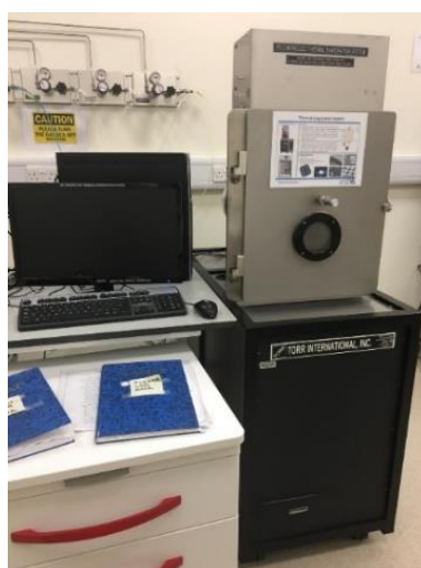
Figure 4.45 Thermal evaporator for Au deposition.
