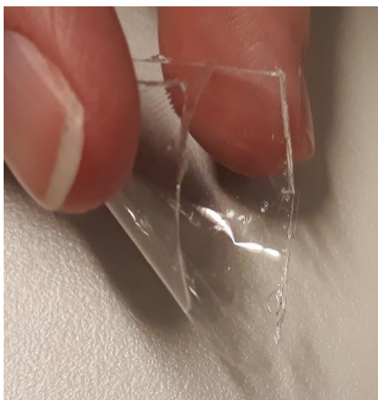
Figure 4.3: Optimised ratio of toluene to PMMA for host material displaying flexible properties
