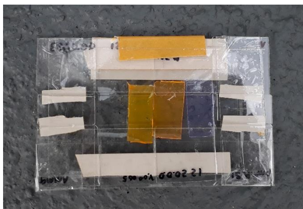
Figure 3.10: Lumogen thin-films. L to R: PMMA, yellow, orange, and violet
