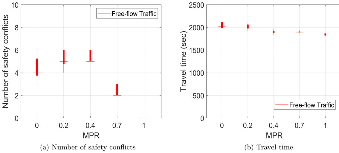
Figure 7.16: Traffic safety and efficiency performance using the MPF IFT-based CAV control in free-flow traffic condition at different penetration rates, with and without packet drops.
