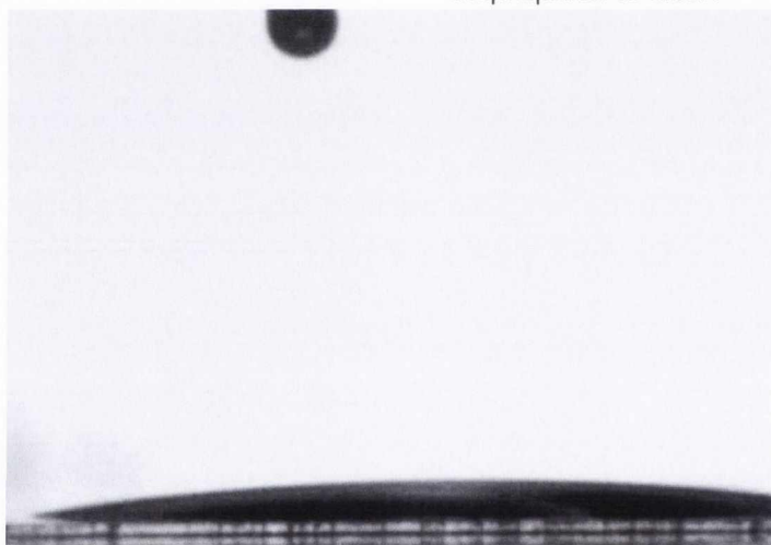
Cleaned by soap/water, acetone sonication, water rinse, methanol sonication, water rinse, N 2 dry and O 2 plasma clean.
