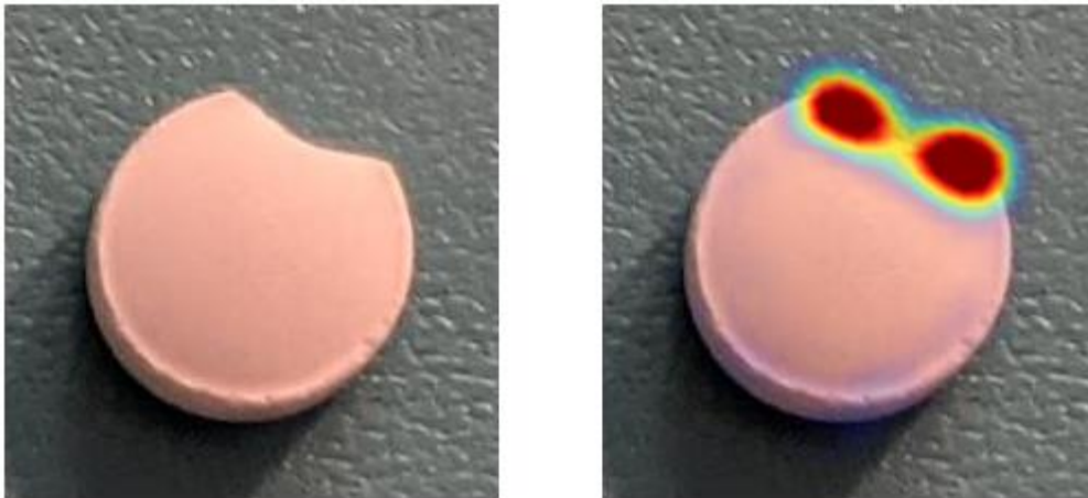
Figure 2.5: Output image from the original Matlab™ tablet anomaly detection code. Original image of a chipped tablet (left) and the same image with applied heat map (right) highlighting the area of the anomaly.
