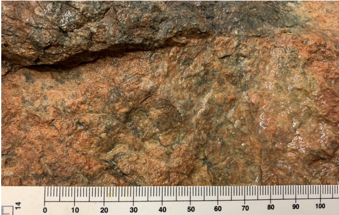
KY05 Salmon pink, coarse grained, qtz + k-feldspar, some chlorite veinlets, foliation/ deformation fabric indicates shearing. Pegmatities. Intrusives.
