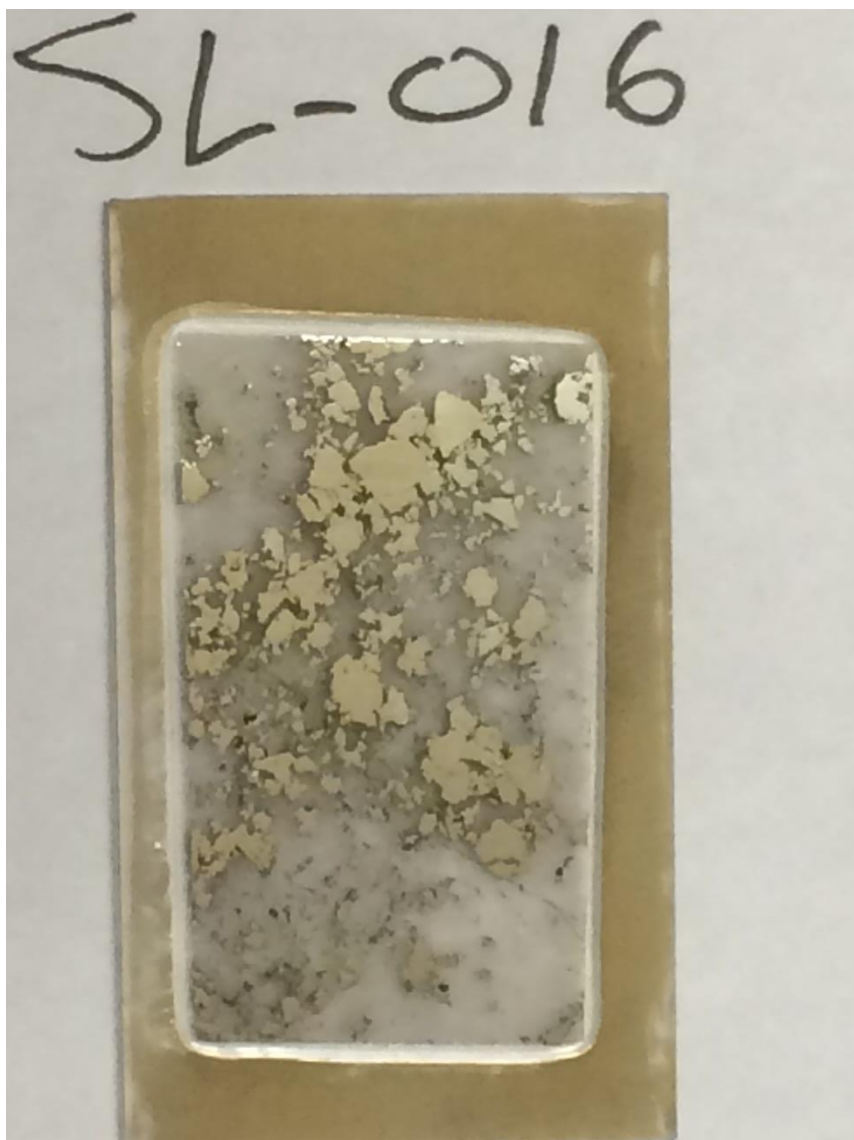
SL16 Unknown sample ID. Polished section is of pyrite with euhedral habit and brecciated texture.
