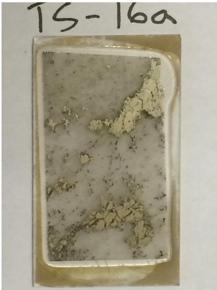
TS16a. Unknown sample ID. Polished section is of pyrite with small disseminations. Internal pyrite texture of possible brecciation
