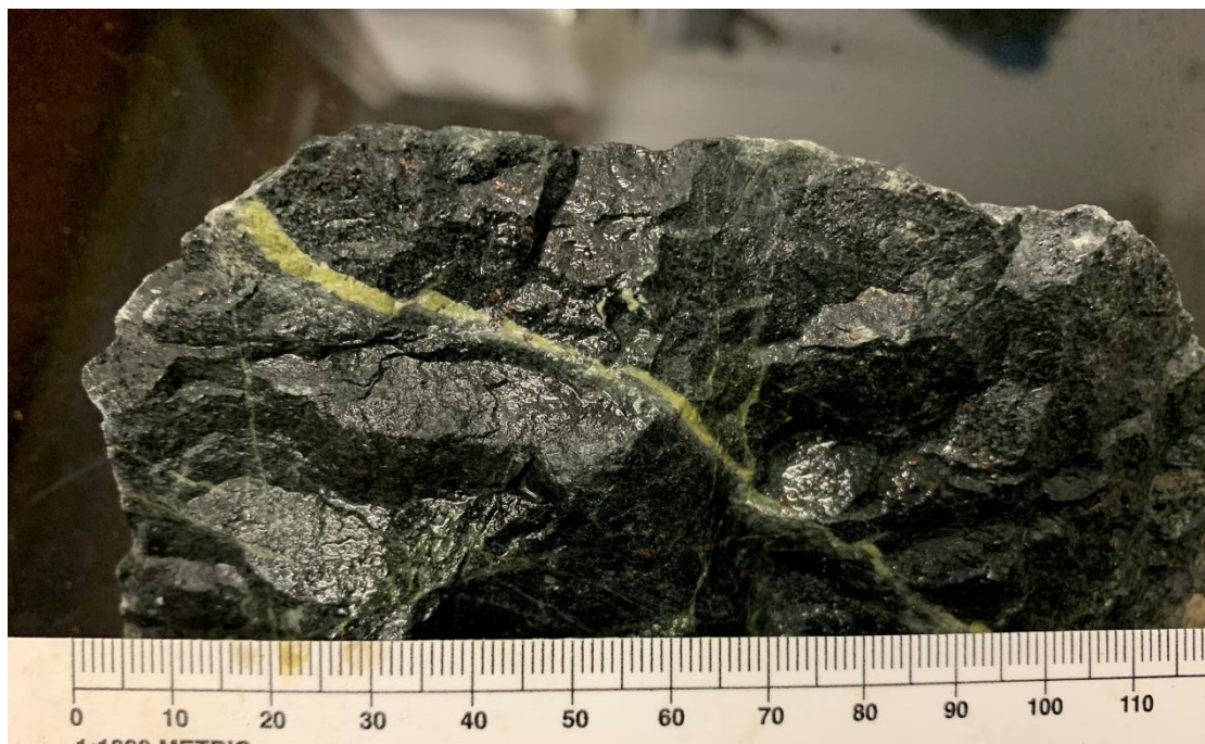
KY02 Black, fine grained, 40-50% qtz, weak chlorite throughout, late green veins - epidote. Dolerite. Upper ophiolite. TPG
