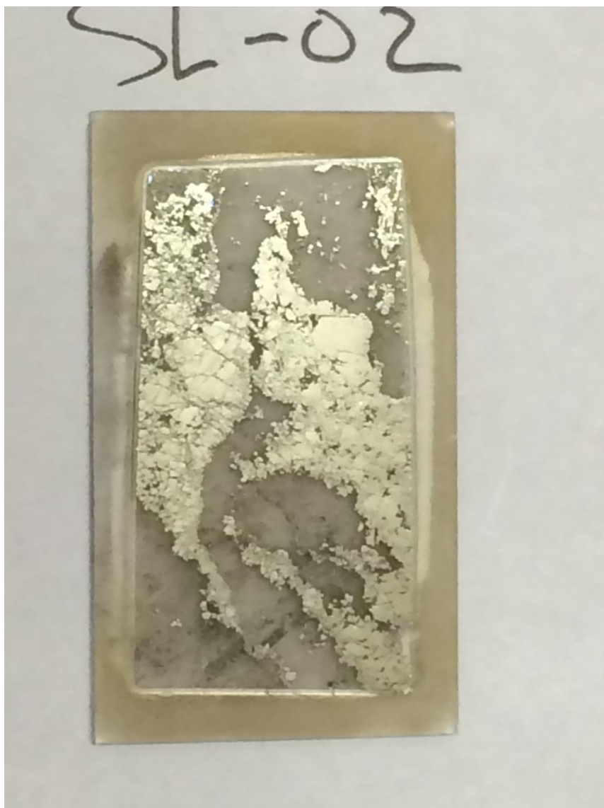
SL02 Unknown sample ID. Polished section of massive pyrite with internal brittle, brecciation texture.
