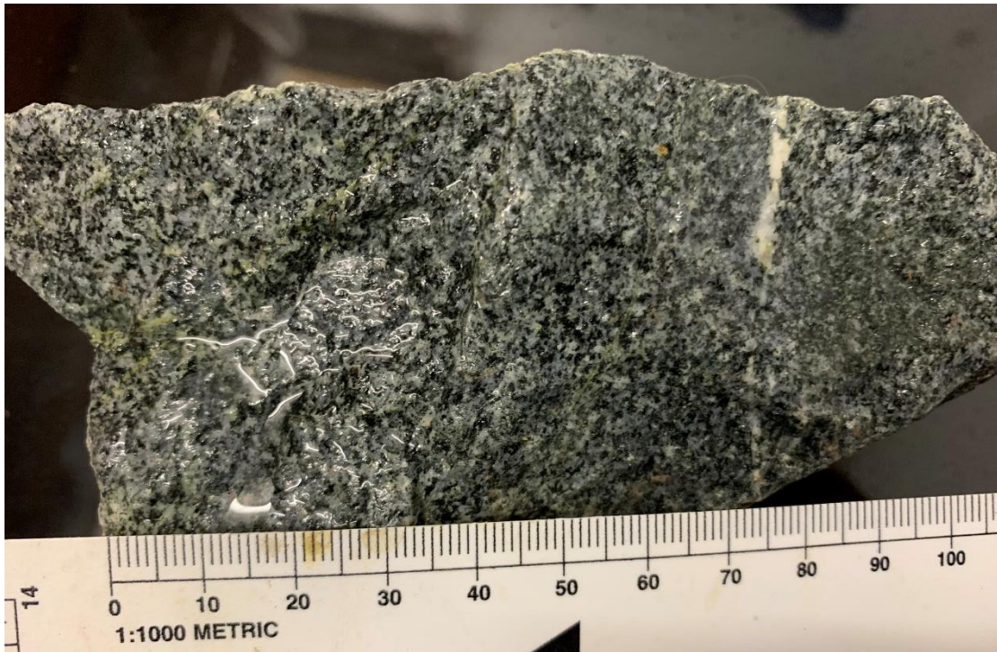
KY01 Grey, medium to coarse grained, 50-60% qtz, isotropic, biotite, minor k-feldspar. Gabbro to microgabbro. Lower ophiolite. Tyrone Plutonic Complex. Orritor Quarry
