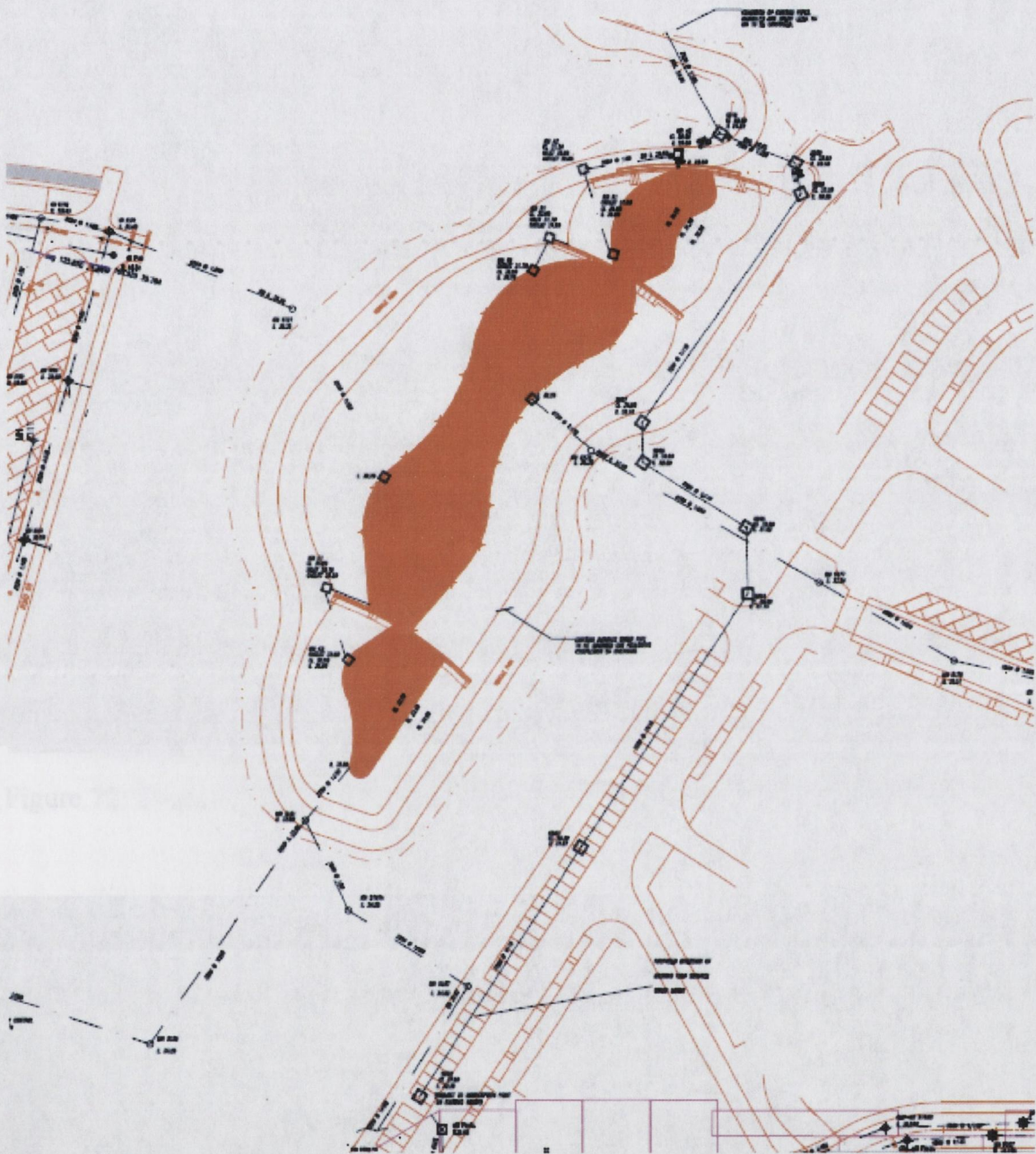
Figure 69: Design drawing of retention pond in Pelletstown from planning files
