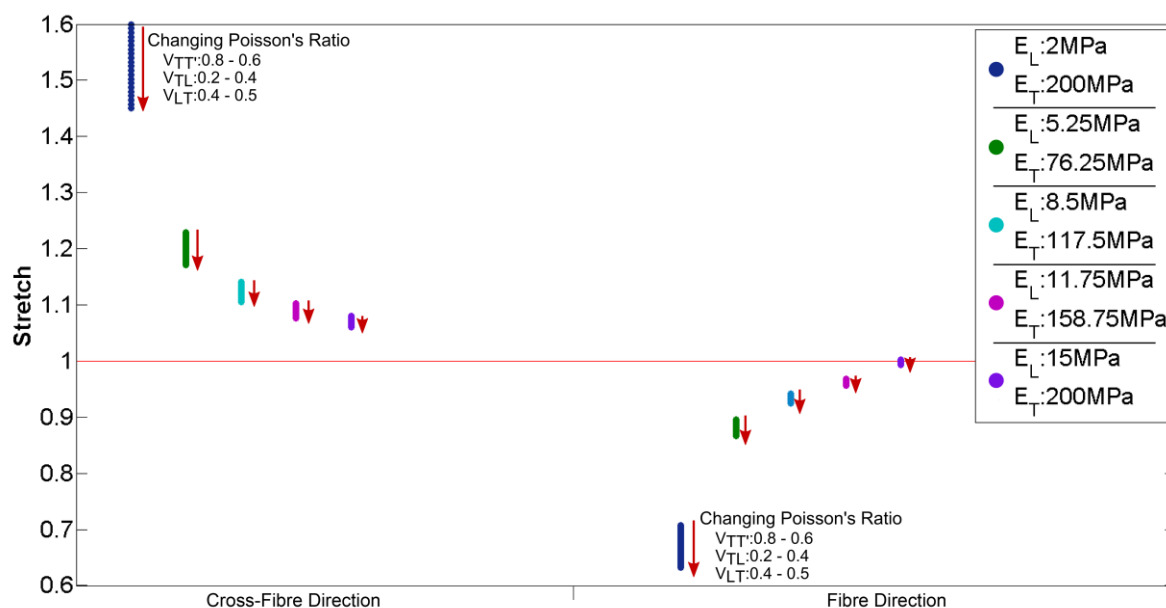
Figure 8.21 – Predicted strains from Hooke's Law analysis in fibre and cross-fibre directions for a range of Poisson's Ratios and Young's Moduli.
