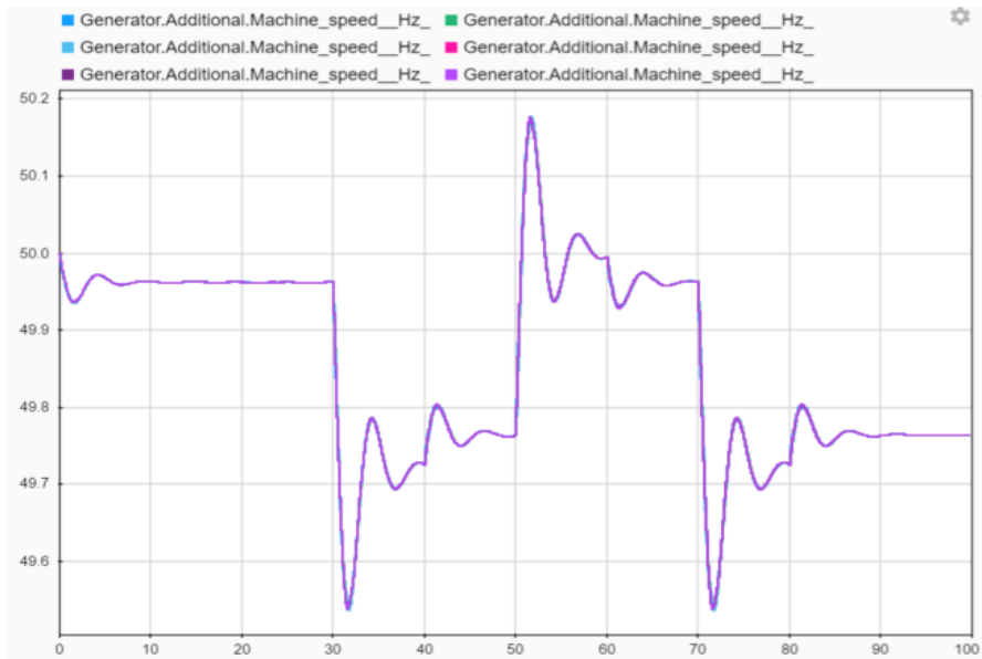
Figure 2-32: Frequency plot of a system experiencing sudden load changes
