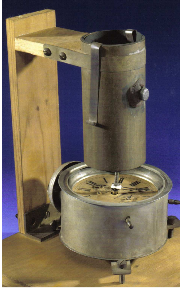
Figure 10. Improved rotation X-ray camera made using a wind-up alarm clock. Gluing to it a nail has extended the spindle. A crystal was mounted at the sharp end of the nail which rotated steadily in the X-ray beam. Bicycle clips were used to hold the photographic film against the inner surface of a metal cylinder. The X-ray beam entered the camera through a porthole half way up the cylindrical chamber.
