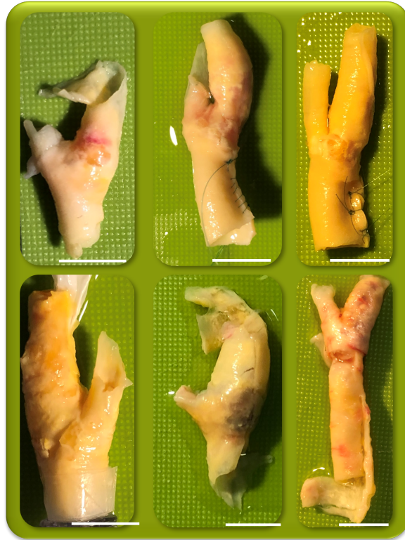
Figure 4.1: Fresh human carotid endarterectomy samples prepared for inflation testing. Scale bars: 1 cm.
