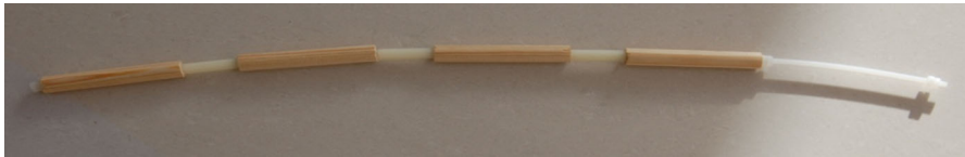
Fig. 3 Rod to measure moisture content at different depths in the wall
