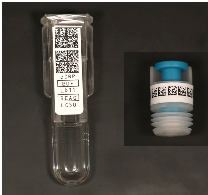
Figure 5.2 Cuvette and reagent cap. Both present with bar code labelling.
