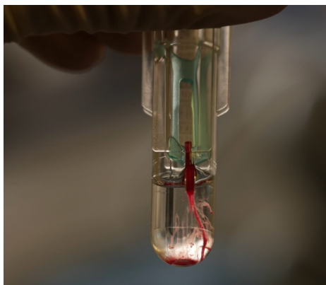
Figure 5.7 The collector is inserted in the cuvette to release the sample. A system of guides and stoppers ensures that the sample collector does not touch and potentially damage the base of the cuvette.
