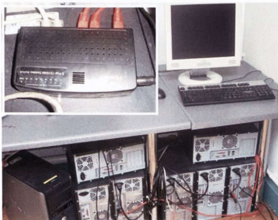
FIGURE 3.13. PERSONAL HPC SYSTEM (MODEM HUB INSERT).
