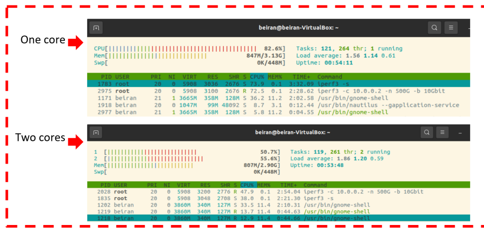
Figure 4.5: CPU Utilization htop measurement for SDN
