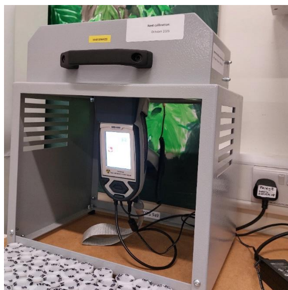
Figure 10.3. X-ray Fluorescence for semi-quantitative measurements for elements.
