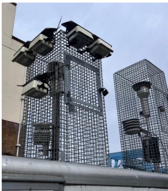
Figure 5.1. Co-location of the devices with EPA monitor at Ringsend (4th to 17th May 2023).
