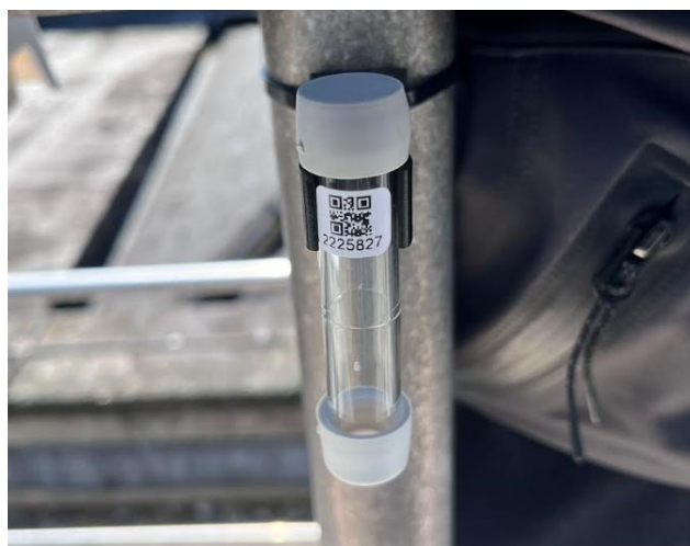
Figure 4.5. Diffusion tubes for passive \text{NO}_2 sampling.
