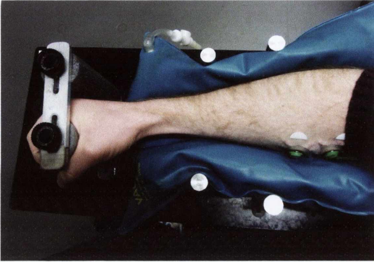
Figure 3.3. The manipulandum used to measure force of wrist flexion during the SIFT. The wrist was secured using vacuum packs and stabilising metal rods. The static handle was attached to a torque transducer.
