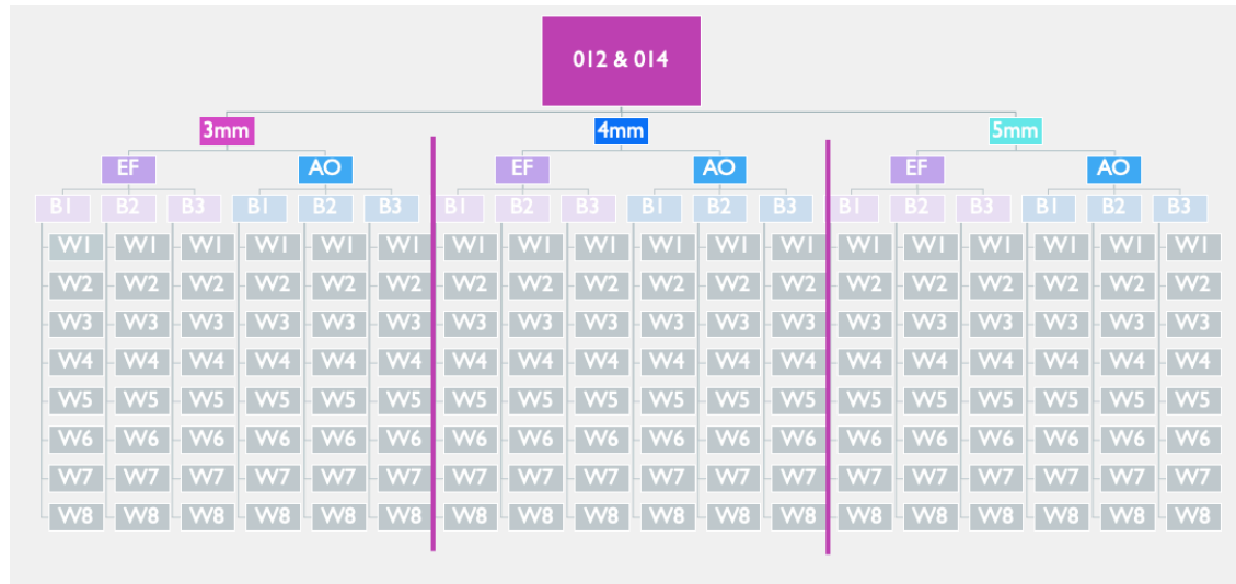
Figure 3.2. Summary of archwire selection. Nickel titanium archwires with diameters of 0.012" and 0.014" were selected. Eight archwires were tested from three batches of two brands (Euroform or American Orthodontics) for displacements of 3-, 4- or 5- mm increments.
