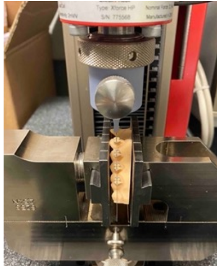
Figure 3.6. Zwick Roell ZwickiLine Z5.0 used for three-point bending test
